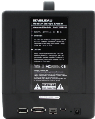
TMSS-IIO1 rear view USB, eSATA, FireWire, MiniUSB, & Power Connectors
